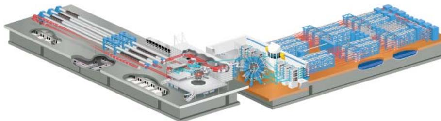
Fig. 1. The OMEGA EP and OMEGA 60 Laser Systems are shown on the left and right, respectively. Each system contains a target chamber for experiments and selected beams from OMEGA EP can be directed to the OMEGA 60 chamber for joint operations
