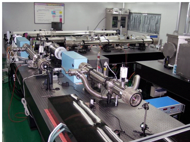
Final amplifier and pump laser
