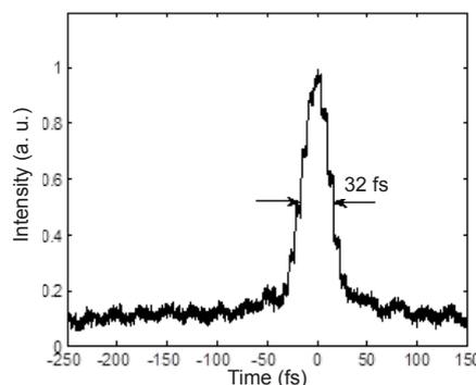
Fig. 4 Measured autocorrelation trace of the pulse
