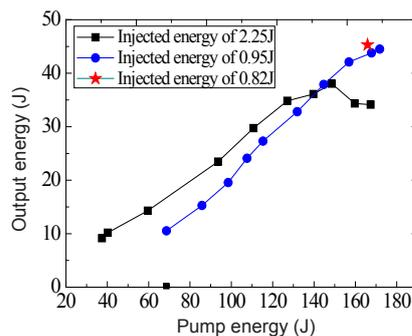
Fig. 3 Output vs pump energy at different injection
