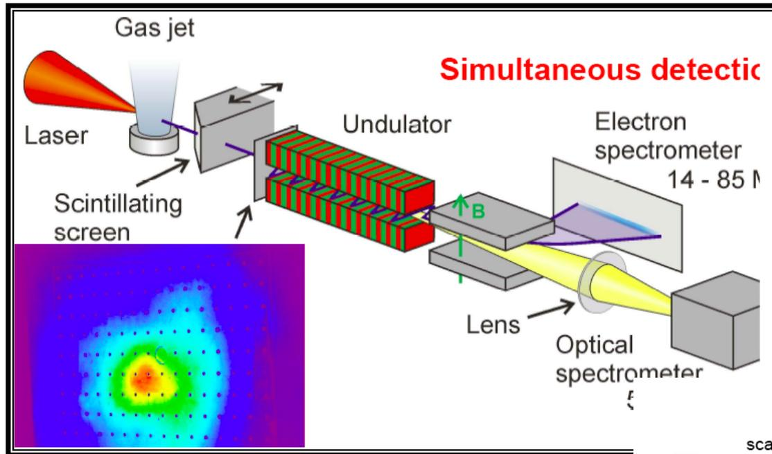
Simultaneous observation of electron and optical spectrum
