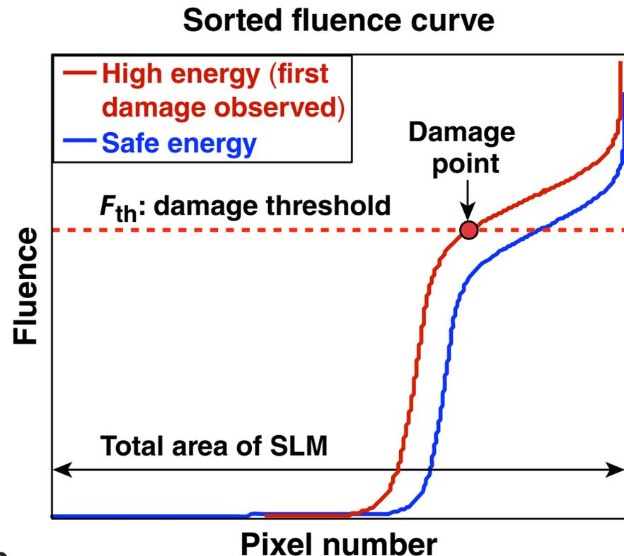
The SLM sample survived 9 h of irradiation (5 Hz) at an apparent energy density of 230 mJ/cm<sup>2</sup>.
