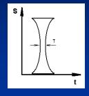
Peak intensity ~ 0.5\*10<sup>12</sup> W/cm<sup>2</sup>, energy of incident pulse – 0.5mJ, bulk of material – 1.2 cm plate of quartz. Pulse compression by factor of 5 (from 92 fs to 19 fs) with a few percent transmission efficiency
