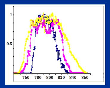
Blue curve (diamonds) represents the spectrum without the glass plate (no SPM), pink curve (squares) – with plate of the 0.8 cm thickness and yellow curve (triangles) – with glass plate of 2 cm thickness.
