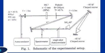
Peak intensity ~ 8\*10<sup>12</sup> W/cm<sup>2</sup>, energy of incident pulse – 0.48mJ, bulk of material – 0.3 cm BK7. Pulse compression by factor of 3 (from 42 fs to 14 fs) with 45 % transmission efficiency
