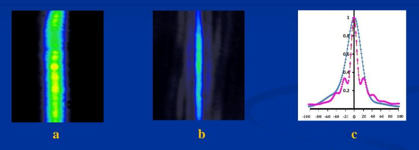
a – autocorrelation picture of the initial transform limited pulse (30 fs), b - compressed
