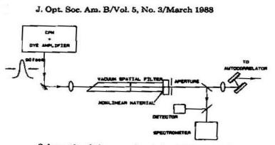
Schematic of the experimental apparatus used for highpower compression.
