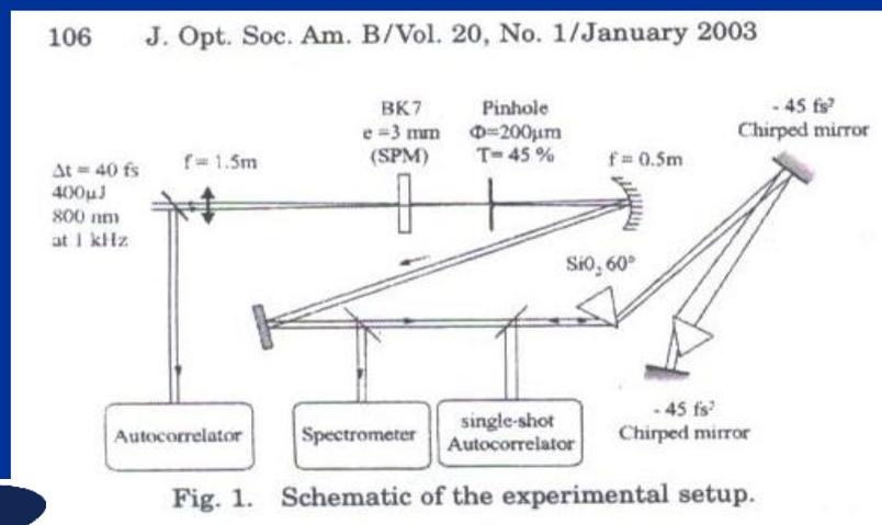
Peak intensity  $\sim 8 \cdot 10^{12} \text{ W/cm}^2$ , energy of incident pulse – 0.48mJ, bulk of material – 0.3 cm BK7. Pulse compression by factor of 3 (from 42 fs to 14 fs) with 45 % transmission efficiency
