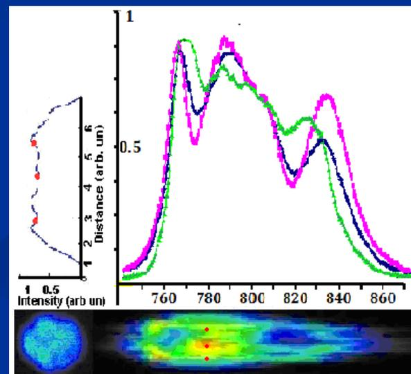
Bottom picture: on the left-output beam of the HERCULES laser, on the right - spectrally resolved beam passed through 2cm glass plate, above: on the left - spectrally integrated spatial energy distribution, on the right - lineout of the spectrum taken at the spatial points shown as red dots.
