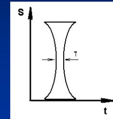
Peak intensity  $\sim 0.5 \cdot 10^{12} \text{ W/cm}^2$ , energy of incident pulse – 0.5mJ, bulk of material – 1.2 cm plate of quartz. Pulse compression by factor of 5 (from 92 fs to 19 fs) with a few percent transmission efficiency
