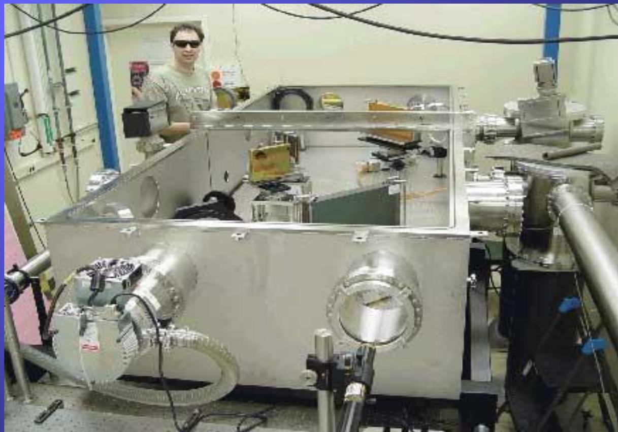
The 6" diameter output beam is compressed to 30 fs pulse duration. To keep the pulse duration at this value +10% during focusing, the precision of the grating alignment has to be not worse than  $10^{-5}$  radians. For this, the beam of the HeNe laser was expanded to 2.5" diameter.
