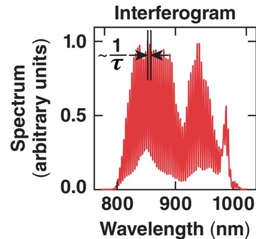
$$\Phi_{\text{MEAS}}(x, y, \omega) = \phi_{\text{NOPA}}(x, y, \omega) - \phi_{\text{REF}}(\omega) - \omega\tau$$
