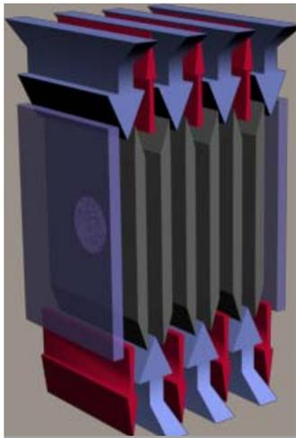
Use of cryogenic gas cooled amplifier heads
