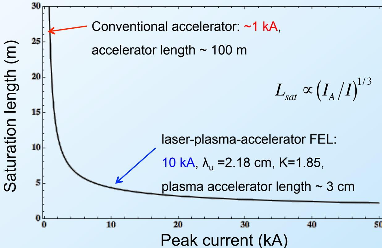
■ Ultra-high peak current  $\Rightarrow$  reduced undulator length for saturation
