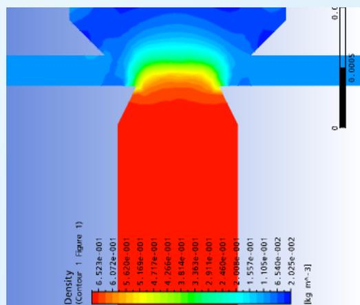
Density profile in capillary obtained from fluid simulation (benchmarked by interferometry)
