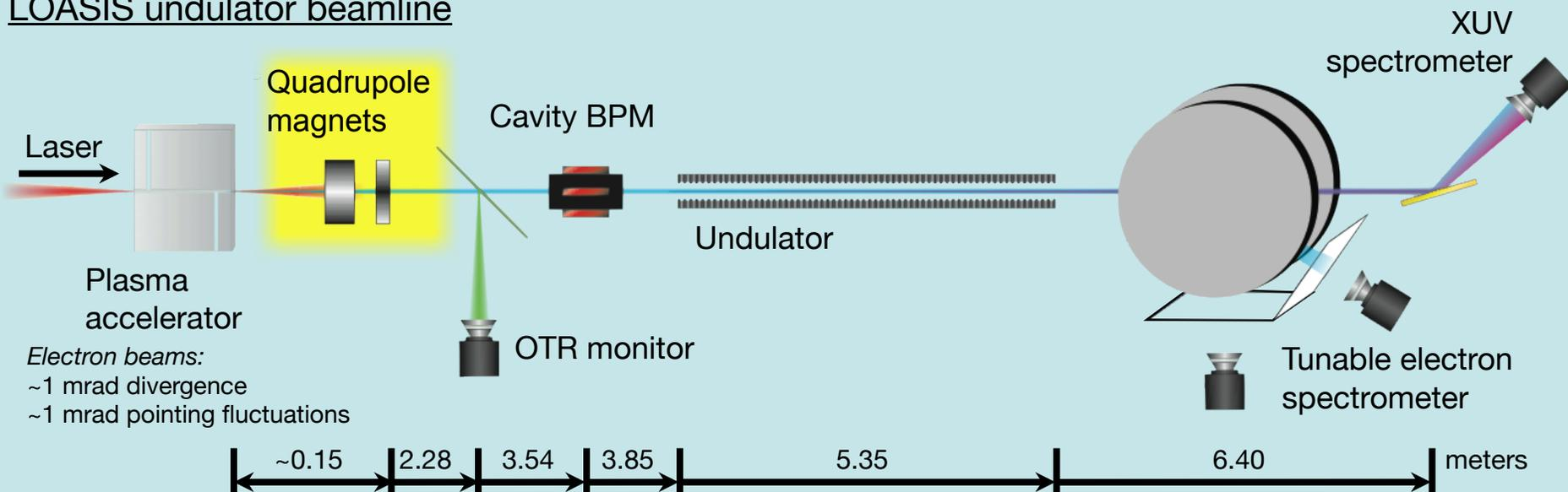
Electron beam transport by quadrupole magnets will allow for
