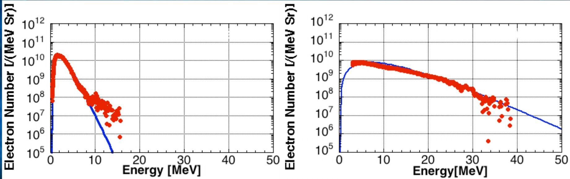
Figure (a) and (b) are the ILE case and the RAL case. In (a), the laser intensity is  $6.43 \times 10^{18}$  W/cm<sup>2</sup>. The target material and thickness are Al and 100  $\mu$ m. In (b), the laser intensity is  $3.16 \times 10^{20}$  W/cm<sup>2</sup>. The target material and thickness are Cu and 25  $\mu$ m.
