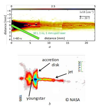
**Fig. 2.** (a) Experimental image [B. Albertazzi et al., Science, 2014] (recomposed from 3 images) of a long, stable plasma jet produced by irradiating a Teflon target by a high-power laser. The jet is magnetically confined by the homogeneous 20 T magnetic field, (b) Hubble space-telescope image of the object HH30
