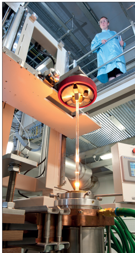
Aiming high A 6-m fibre drawing tower at the University of Southampton's Optoelectronics Research Centre is used to create the components that are required in a fibre laser.
